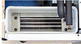
Innovative finned coil evaporator with high efficiency.
